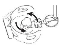
2. Turn the valve on the tank completely counterclockwise to the OPEN position.
