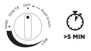
CLOSE tank valve and turn control knob to OFF position. Wait at least 5 minutes for gas to completely dissipate before attempting to manually light. Do not light if you smell gas.
