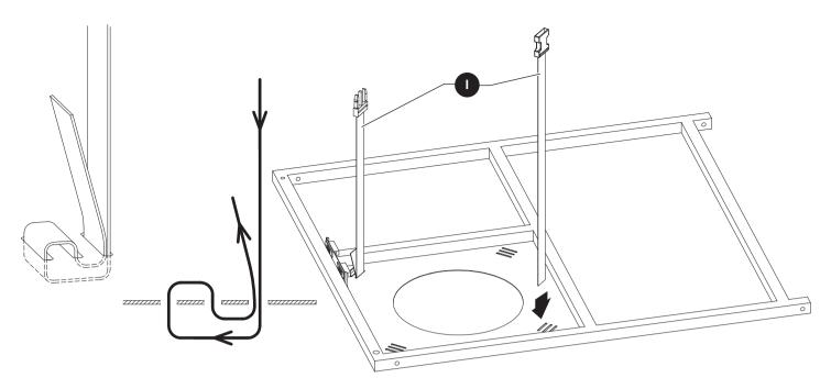
5. Thread each half of the tank strap into the slots in the bottom plate as shown. Pull the strap snug.
