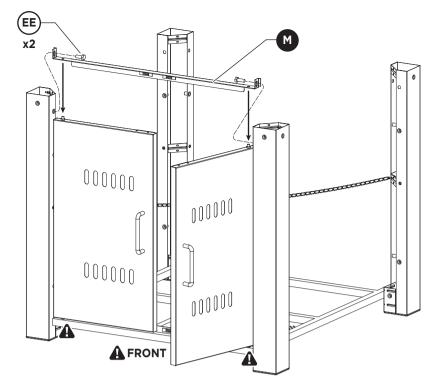
8. Position both doors in the opening between the front legs. Insert the pins on the bottom of the doors into the matching holes in the bottom plate.
