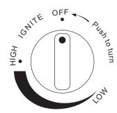
1. Press and turn control knob clockwise to OFF position. The burner may make a slight popping sound as it extinguishes.
