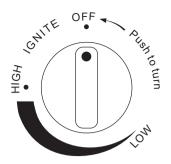
1. Ensure the control knob is in the OFF position.
