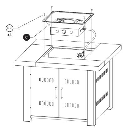
**11.** Insert the burner assembly by aligning the holes with those in the table. Attach with hardware shown.
