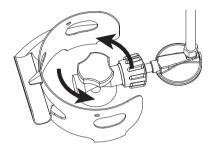
2. Turn the valve on the tank completely counterclockwise to the OPEN position.
