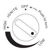
4. Hold the control knob down (for no more than 10 seconds) until the burner ignites. When the burner lights, release the control knob.
