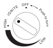
3. Press and turn the control knob counterclockwise to the IGNITE position or until you hear clicking sounds.
