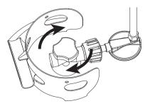
2. Turn the tank valve completely clockwise to the CLOSE position. If not using this appliance for an extended period, also disconnect the gas hose/regulator from the tank.
