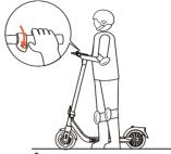
Do not press the throttle when walking with the scooter.
