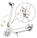
2. Unfold the stem and fasten the folding wrench. Make sure the unlocking key springs up normally after fastening. Be sure to buckle up properly.
