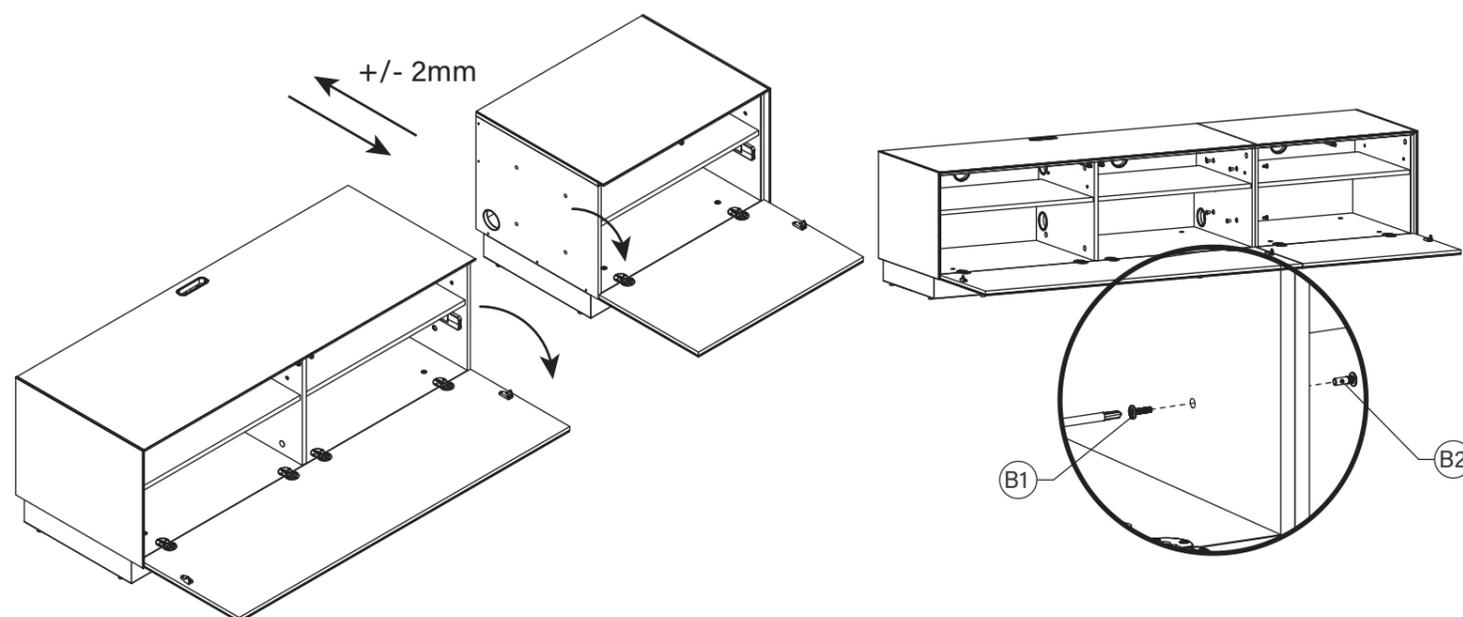
ADJUSTING LEVEL OF DRAWER FOR D/FD/DD VERSIONS
