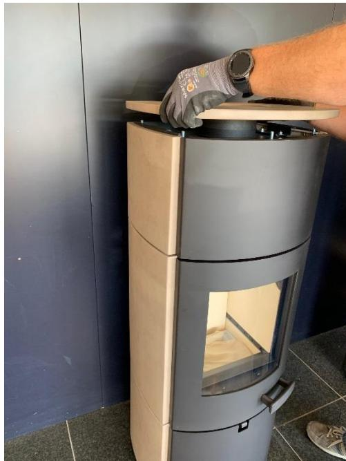
13. Now carefully place the ceramic top plate on the stove. By adjusting the threaded pins, the plate can be aligned with the aid of a slotted screwdriver
