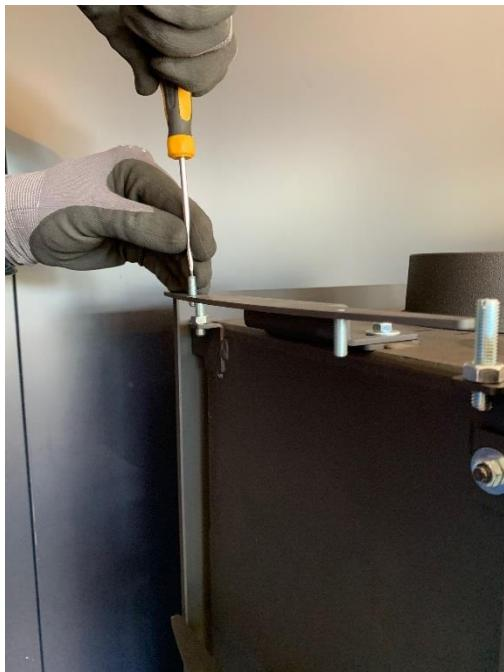
6. Now screw two setscrews (M5 x 20) into the upper ceramic holder until they are flush with the upper side.
