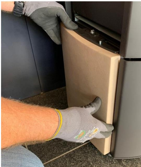
9. Align the ceramic so that a gap of approx. 3-5 mm is created. Now tighten both the screws of the lower and upper ceramic holder.
