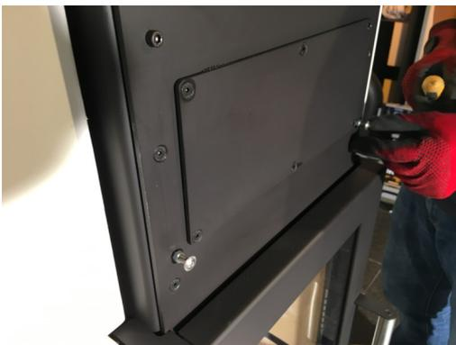
23. If the front plate has to be aligned vertically, the spacer screws in the stove's front plate can be screwed in or out accordingly. When the correct position is found, the position of the screws is secured by tightening the nuts.
