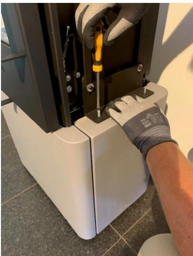
9. Screw two set screws (M6 x 30) into the threads provided until they are about halfway into the lower tile.
