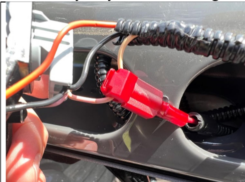
Plug red power extension wire into the wire tap.
