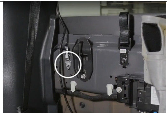
Attach black ground wire to the 8mm stud circled above.
