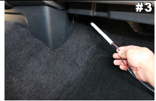
Route driver side lamp behind center console toward driver side.
