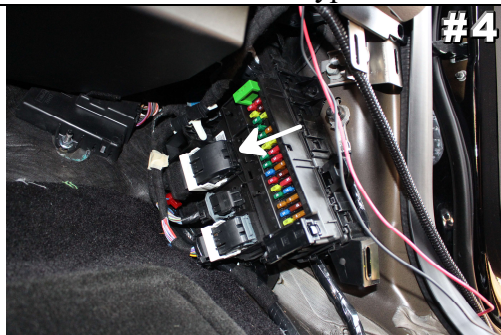
2015+ Locate largest connector with white bar – it is 3rd from the bottom.
