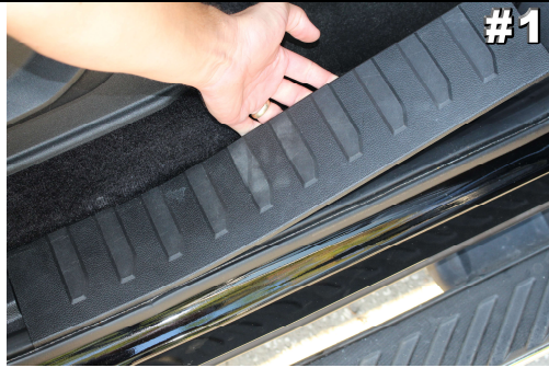
Remove passenger side door sill plate carefully.
