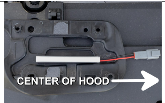
2 Mount LED as shown on backside of retention plate. 3
