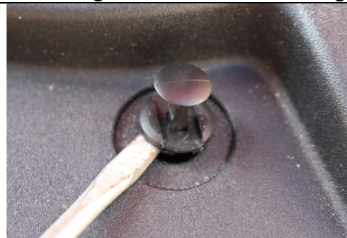
7 Pry up on center part of pin first. Then pry out entire retainer pin.
