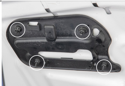
1 Remove the 4 – 9mm nuts that secure the retention plate.
