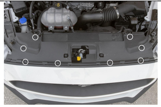
5 Remove radiator cover shown. Save the 8 retaining pins. 6
