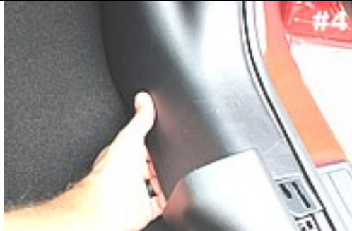
Remove kick panel shown. First pull upward, then backward gently.
