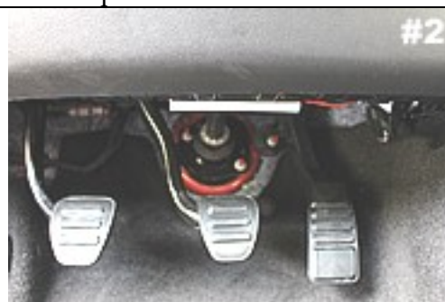
Shown is the LED lamp centered under driver side of dash.
