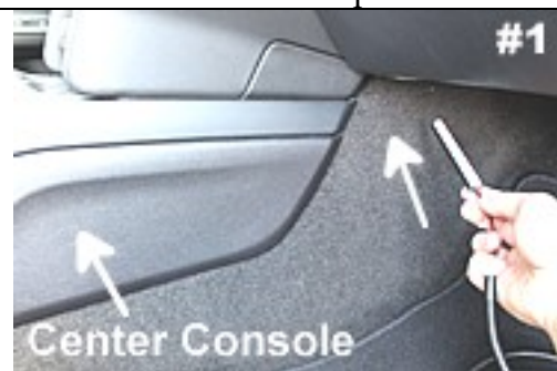
Route DS lamp behind center console to driver side.
