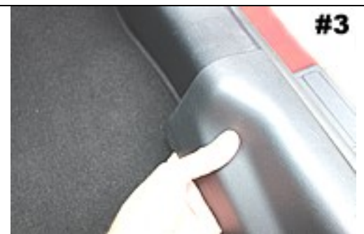
Loosen passenger side door sill plate – you may remove if desired.
