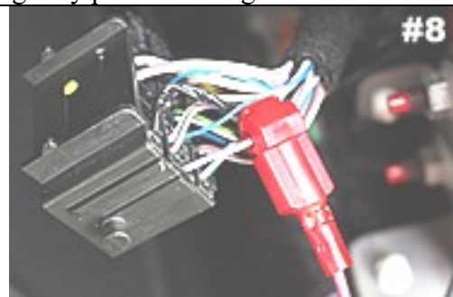
Plug red wire into the wire tap.
