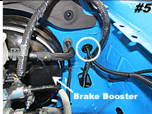
Cut small "X" in grommet and route wiring through the hole.
