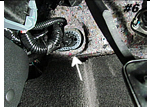
Cut small "X" in boot and route wiring through the hole.
