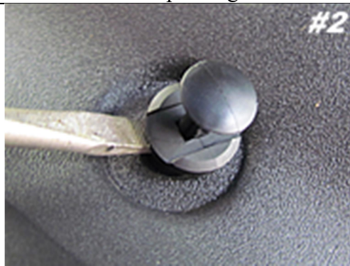
Pry up on center part of pin first. Then pry out entire retainer pin.
