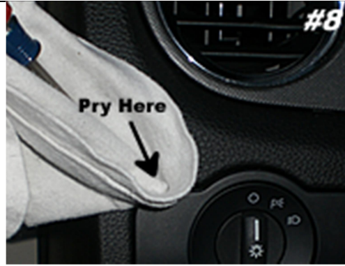
Pry up gently to loosen switch panel.
