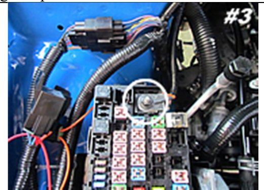
Be sure that the bolt is re-attached tightly enough that it will not loosen.
