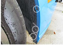
Remove 3 bolts on driver and passenger side wheel well.
