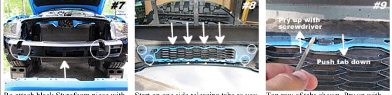
Re-attach black Styrofoam piece with 4 ribbed push pins before continuing.
