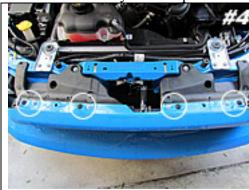
Remove 4 bolts (8mm) and 4 pushpin Phillips screws.
