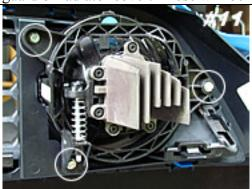
3 screws hold on each fog lamp. Use 5/16 socket or flat head to tighten.
