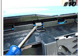
Top row of tabs shown. Pry up with screwdriver while pushing tab down.
