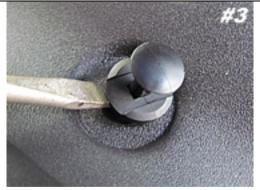
Pry up on center part of pin first. Then pry out entire retainer pin.
