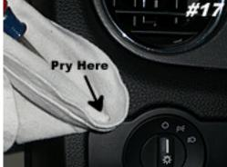
Pry downward slightly. Be gentle and Pry up gently to loosen switch panel. cautious when doing so.
