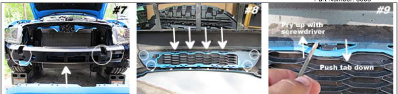
Re-attach black Styrofoam piece with 4 ribbed push pins before continuing.
