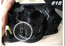
3 tabs hold switch in. One of the tabs is circled in the picture above.
