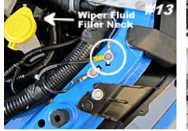
Attach ring terminal to bolt circled above. Firmly re-tighten the bolt.
