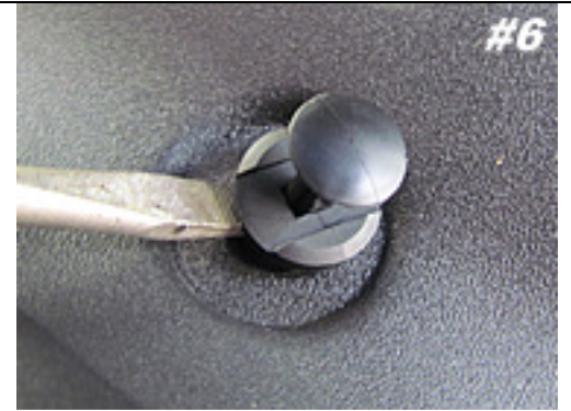
Pry up on center part of pin first. Then pry out entire retainer pin.
