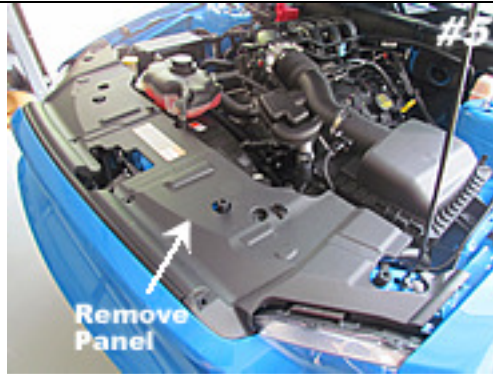
Remove black panel shown. Save 8 retaining pins for re-install later.
