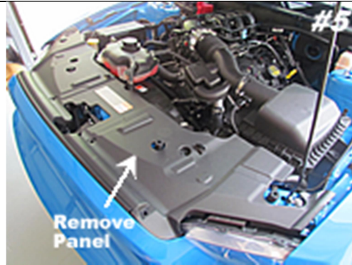
Remove black panel shown. Save 8 retaining pins for re-install later.
