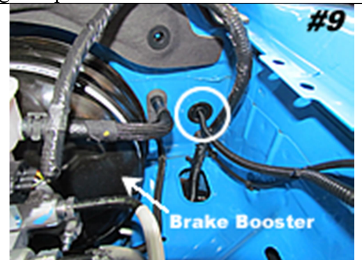
Cut small "X" in grommet and route wiring through the hole.
