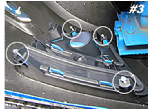
New bezel locks into place with 5 tabs and is secured by 4 screws.
