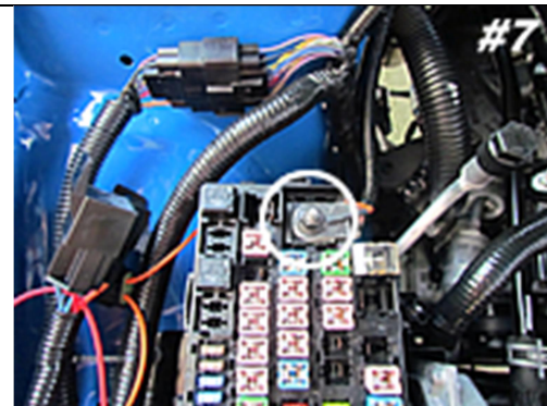
Be sure that the bolt is re-attached tightly enough that it will not loosen.
