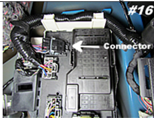
Connect to white wire on connector shown above using a wire tap.
