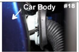
Loosen connector by depressing top & bottom tabs and pulling ½ inch out.
