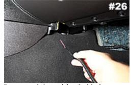
Pass remaining wiring behind center console to drivers side.
