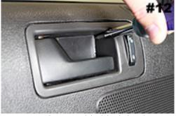
Remove trim panel behind the door handle with flat head screwdriver.
