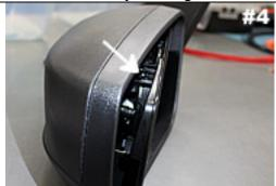
Shows top retaining tab. Insert flat head screw driver here to release tab.
