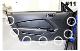
Remove screws around perimeter of door with 7mm driver.
