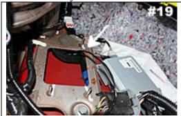
Shown is the driver side where the puddle lamp wiring comes through
