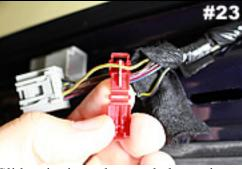
Slide wire into place and close wire tap firmly.
