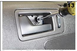
Remove the T30 screw with a Torx driver.
