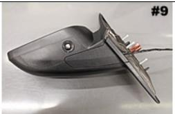
Mount the lamp using the white nut provided, then route wiring as shown.
