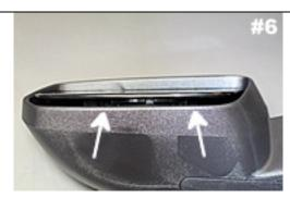
Bottom view of Drivers side mirror. Shown are 2 of the retaining tabs.
