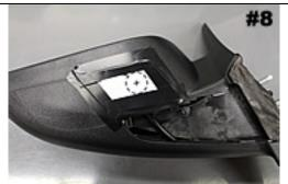
Bottom of driver side lamp with drilling template attached.
