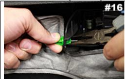
Use a pair of needle nose pliers to remove door handle cable.
