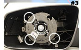
3 Retaining tabs (circled) hold the mirror glass in place.
