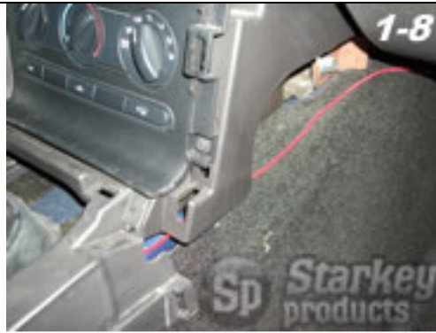
Route red wire towards glove box. Then re-install trim panel.
