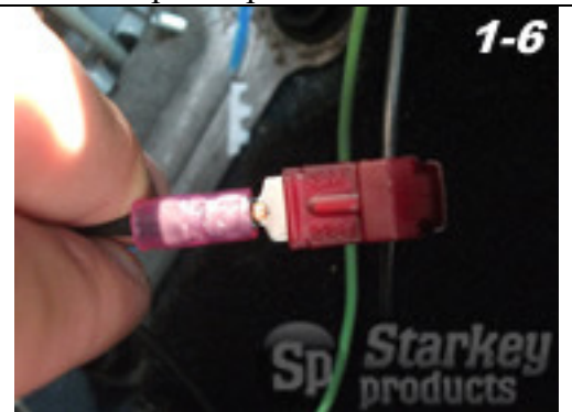
Plug correct wire into the wire tap as indicated above.
