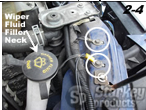
You may attach the ground wire to either bolt in the picture above.
