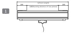
Step 1: Measure the product's total length L and calculate the installation distance LA of the two mounting plates.
