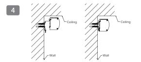
Step 4: Hang the product on the hanging board (as shown in the figure above) and tighten the M3x16 screws. If the product needs to be moved left and right, loosen the M3x16 screws to move the product to the desired position.
