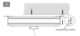
**Step 3:** Knock the plastic granules into  $\phi$ 8 holes (plastic parts do not stand out the ceiling plane), move both ends of the product top mounting plate to close to the product plastic end cover (as shown in the figure above), two M6 screws through the installation holes, screw into the plastic granules.
