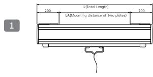
Step 1: Measure the product's total length L and calculate the installation distance LA of the two mounting plates.
