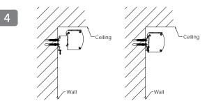
Step 4: Hang the product on the hanging board (as shown in the figure above) and tighten the M3x16 screws. If the product needs to be moved left and right, loosen the M3x16 screws to move the product to the desired position.
