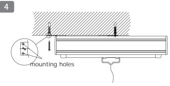
Step 4: Parallel move the product, align the mounting hole at the other end with the glue particle (as shown in the figure above), and tighten the M6 screw.
