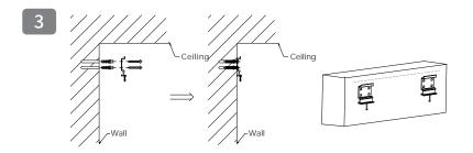
Step 3: Hammer  $\phi 8$  colloidal particles into 8 holes (the plastic-free part of the colloidal particles is exposed) M5 self-tapping screws are inserted into the  $\phi 8$ mm colloidal particles through the hole of the hanging plates (the two hanging plates are parallel to a horizontal plane, as shown in the figure above).
