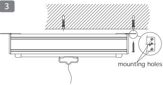
**Step 3:** Knock the plastic granules into  $\Phi$ 8 holes (plastic parts do not stand out the ceiling plane), move both ends of the product top mounting plate to close to the product plastic end cover (as shown in the figure above), two M6 screws through the installation holes, screw into the plastic granules
