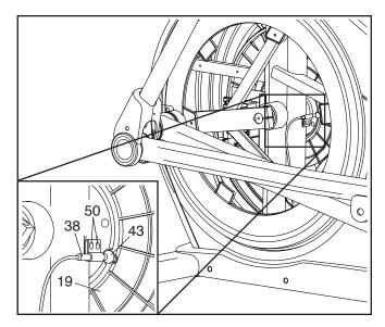
Next, slightly loosen the indicated two M4 x 12mm Self-tapping Screws (50). Slide the Reed Switch (38) slightly closer to or away from the Magnet (43), and then retighten the Self-tapping Screws.
