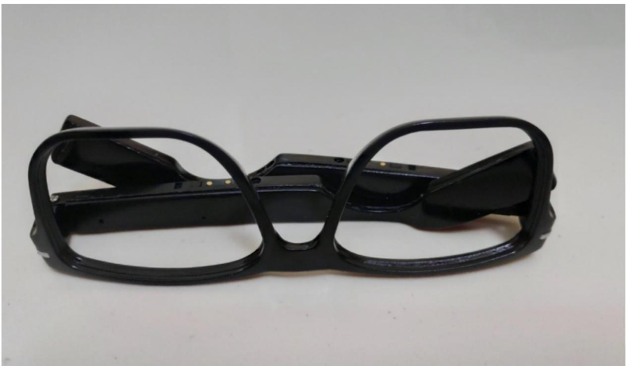
The glasses will power off in these two upside-down positions after 10 seconds. To turn it back on, pick up the glasses and touch the touch area on both temples.
