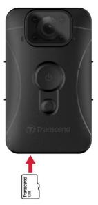
1. Insert a microSD memory card into the card slot on the bottom of the camera.
