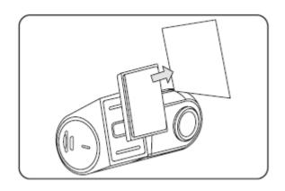
Tear off the film from the detachable adhesive base and fix the device in the proper installation location
