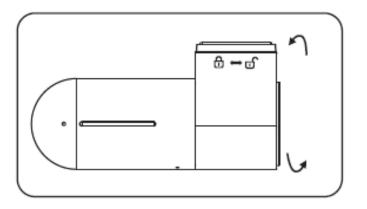
Rotate the cylinder part of the device to adjust the camera angle, and tilt the lens slightly downward so that the camera view is parallel to the horizontal ground.
