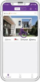
If the camera was not added successfully, hold the reset button for 5 seconds and do it again. Make sure to provide CORRECT WiFi hotspot and password. (2.4G WiFi only)
