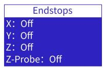
This function can be used for fault diagnosis of endstops and proximity sensor. If the endstop and proximity sensor fail, the state will not change.
