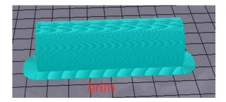
• **Skirt Line Count:** Sets the number of anti-overflow lines at the end of the model in contact with the build platform.
