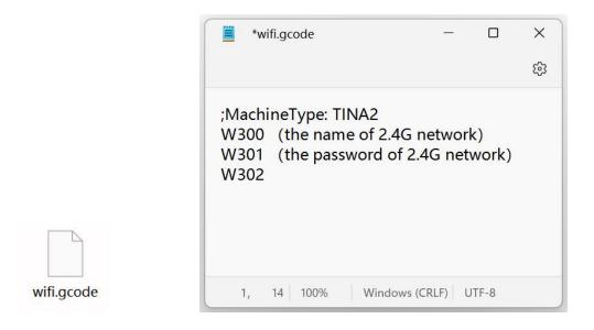
2. Insert the TF card into the TINA2 and choose to print the "WIFI.gcode" file. After few seconds, the info screen show the IP address, which means the network configuration is successful.
