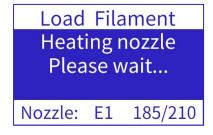
The nozzle will be heated to 210°C, then the extruder will feed the filament to the nozzle. During heating or extrusion, you can press the knob button to exit the current operation.
