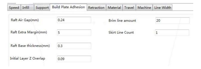
• Raft Air Gap (mm): The distance between the raft and the model. This determines the difficulty of removing the raft from the model.
