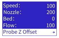
1. Select "Speed", turn the knob to reach the desired speed, and press the knob to confirm.
