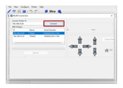
NOTE: IF YOU STILL CANNOT CONNECT TO THE 3D PRINTER, PLEASE CHECK WHETHER THE FIREWALL OF THE COMPUTER PROHIBITS THE SOFTWARE FROM NETWORKING, AND WHETHER THE COMPUTER AND THE 3D PRINTER ARE IN THE SAME LOCAL AREA NETWORK.
