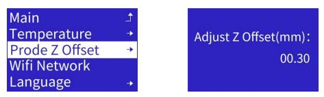
Turn the knob, the nozzle will adjust the height of the printing position up and down. Press the knob to confirm and save.
