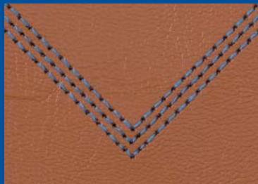
Sewing speed: 2,800sti/min, stitch length: 4mm
