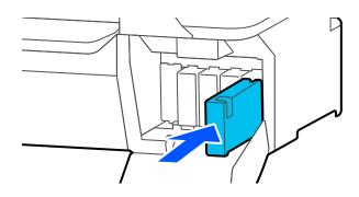
**Note:** Make sure to insert the cartridge into the correct color location
