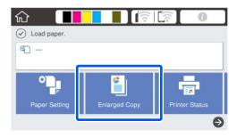
**Note:** If you do not see the **Enlarged Copy** option, make sure the cables connecting the printer and scanner are secure and the scanner is turned on.
