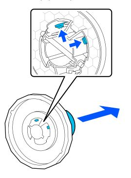
• **3-inch roll core**: Install the 3-inch core adapters on both paper stops. Align the triangle marks on the paper stop with the triangle marks on the adapter and push the adapter in until the tabs are secured.
