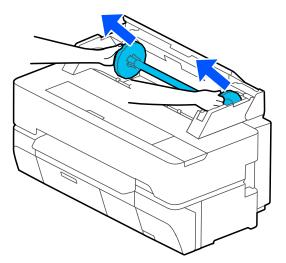
5. Remove the transparent paper stop from the spindle.
