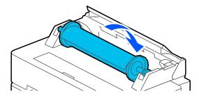
12. Insert the leading edge of the roll paper into the paper feeder until you hear a beep.
