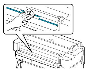
4. Using the cleaning kit or the clean side of the soft cloth, thoroughly wipe the glass surfaces shown below:
