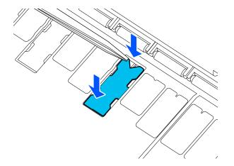
**Caution:** Make sure that no part of the borderless pad extends above the surrounding surface. The borderless pad may rub against the print head and damage it.
