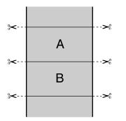
• **Double Cut**: Increases the space between each image and trims each print individually, providing the cleanest edge for borderless printing.
