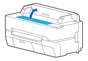
4. Using a soft cloth to remove dust and dirt from the platen. Thoroughly clean the area shown in blue in the image below. Wipe from the inside to the outside of the platen to clean it as shown here.
