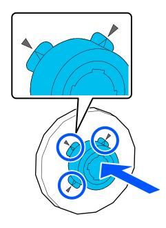
7. Insert the spindle into the roll paper core as shown, with the lead edge of the roll paper facing as shown.
