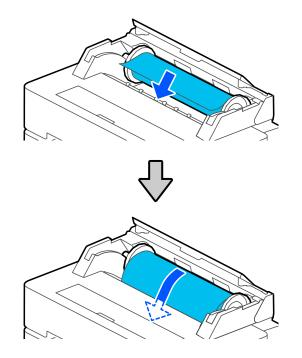
**Note:** Make sure the leading edge of the roll paper is not bent or skewed, or a paper jam or skew error may occur.
