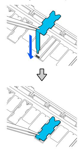
8. Push the protrusions on the sides of the borderless pad into the grooves on the left and right.
