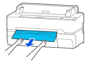
5. Open the front cover and remove any other jammed paper as necessary.
