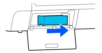
**Note:** Repeat the above procedure for the second maintenance box on the SureColor T5470/T5470M, if necessary. If you are only replacing one of the maintenance boxes, make sure it is the correct one.
