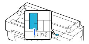
If you are loading an original using the carrier sheet, align the right edge guide with the carrier sheet line:
