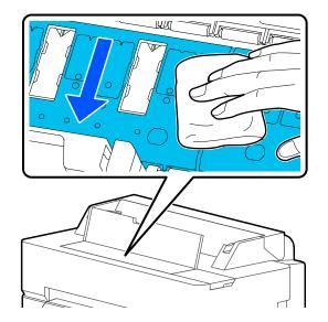
**Note:** For stubborn dirt, dampen a soft cloth with neutral detergent and wring it out, then clean the platen as shown above. Dry the platen with a soft, dry cloth when you are finished.
