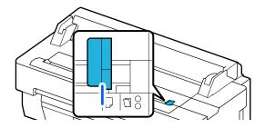
2. Insert the top edge of the original into the scanner slot as shown below. Align it with the right edge guide. Continue inserting the original until you hear a beep.
