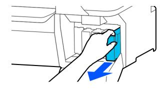
5. With the label facing you, slide the new ink cartridge all the way into the slot.
