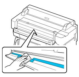
5. Close the scanner cover immediately after you have finished cleaning.
