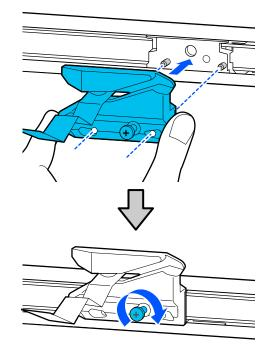
Note: Make sure the screw is tightened securely, otherwise the cut position may shift slightly.
