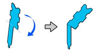
7. Insert the leg of the borderless pad all the way into the hole.
