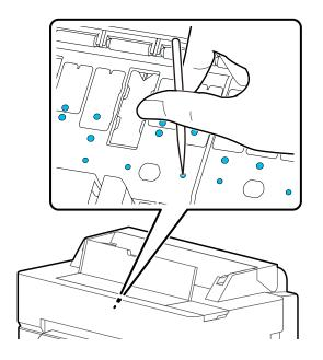
6. Remove any paper particles or dust around the outer edges of the borderless pads using cotton swabs.
