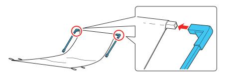
Insert the end of the rods into the front legs of the stand until they snap into place.
