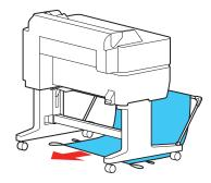
Attach the basket loops to the hooks on the stand as shown.
