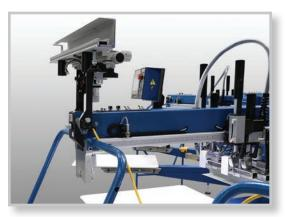
Pneumatic-locking, Quick-Flip™ front frame holders
