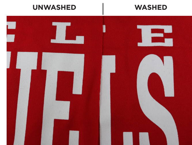
The most obvious failure will be print cracks and most of the time you will see these after 1 wash
