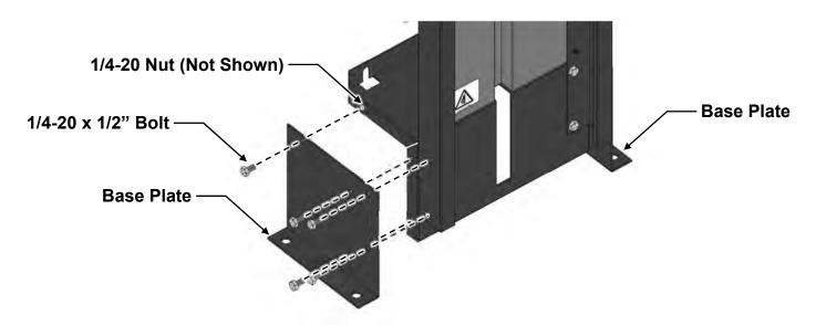
**1)** Remove the existing base plates by removing (10) 1/4-20 x 1/2" bolts and nuts from each side of the machine. Set hardware aside.
