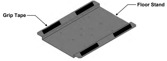
**4)** Install the Floor Stand on to the bottom of the C-1000 using (6) 3/8-16 x 3/4" bolts, washers, and nuts.
