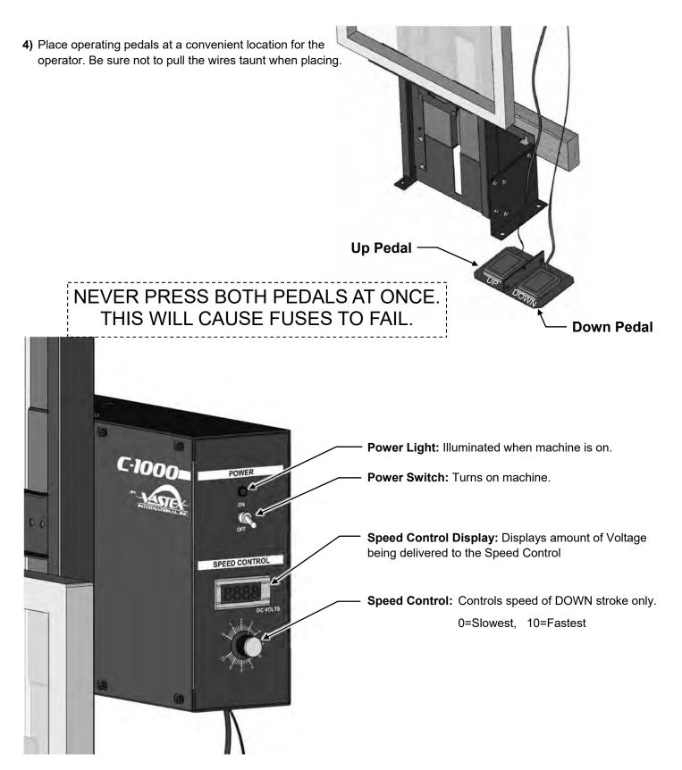
5) After reading and comprehending this manual in it's entirety, plug the machine in to begin operation. See **Page 2** for electrical requirements.
