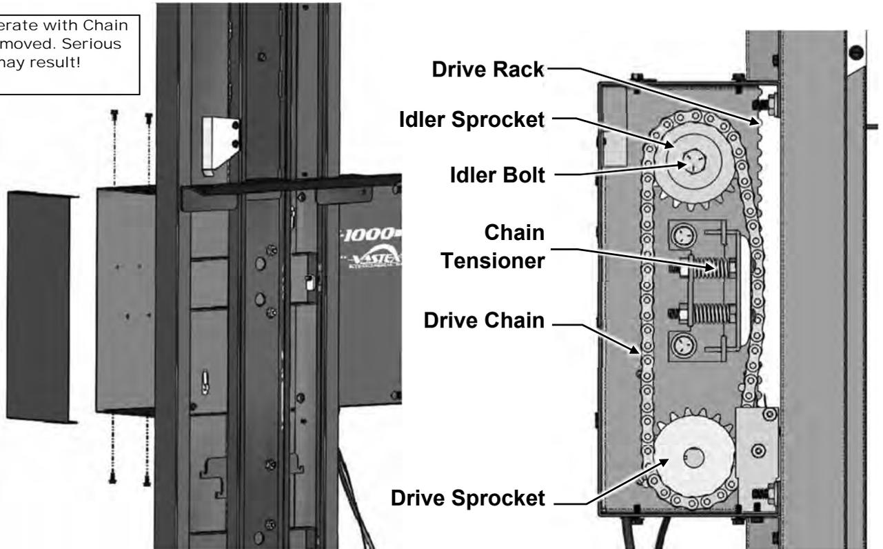
**Access** drive chain by removing (4) #8 sheet metal screws using flat blade screwdriver or 1/4" Nut driver. Then remove Chain Guard.
