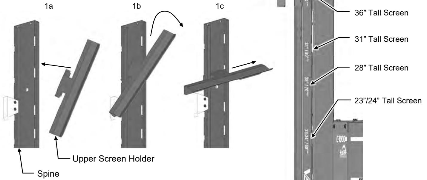
2) Install Scoop Coater Holder in the notch above the screen size you are using. The Scoop Coater Holder is installed the same as the Upper Screen Holder.
