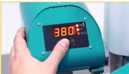
Press MODE once to change the TEMPERATURE. While SET and TEMP are illuminated, press (+) and (-) buttons to adjust the TEMPERATURE.
