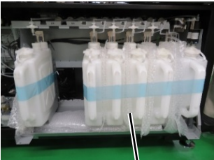
Cushioning material between tanks
