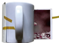
3. Fixing the image on the mug with high temperature tape.
