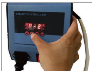
9. Once you have both time and temperature set up. Press OK again to confirm all the setting data. The machine start heating up.
