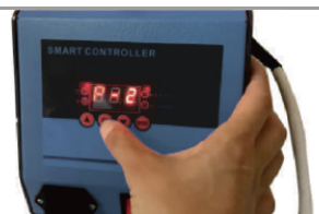
8. Pressing "OK" (the third time) and the screen shows "P-2", you need to set time by press "▼" "▲" (eg.120s). ps: the temp and time will be vary according to the material you use, test it before you do volume production.
