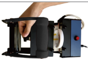
5. Closing the handle and adjust the pressure knob to make sure the mug is well-pressed.
