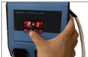
6. Connecting the power cord and turn on the power switch. The display screen should illuminate. Pressing the "OK" key, the screen shows "P-1", you need to set a working temp by press "▼" "▲" (eg.360°F).
