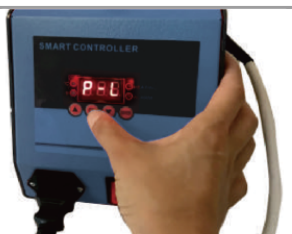
7. Pressing "OK" again and the screen shows "P-L", you need to set a protective temp by press "▼" "▲" (eg.250°F).
