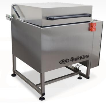
M&R's Qwik-Klean™ automates the highly labor-intensive, tedious process of cleaning squeegee holders and floodbars. Qwik-Klean achieves outstanding results through the combination of a high-volume spray and a rotating squeegee/floodbar holder assembly all within a single chamber. The addition of a final freshwater rinse eliminates the need for post-cycle washing and the possibility of squeegee degradation from chemical exposure.
