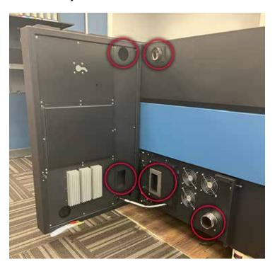
As the door is opened for daily maintenance, check this opening for a build-up of oil. Oil should be drained into a bucket through the spout if you see any build-up. This residue is not drain safe and should be disposed of in cooperation with your local environmental guidelines.
