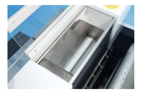
The powder box is equipped with a heating tube, which is automatically energised when the machine is switched on to keep the hot melt powder dry.
