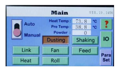
When using Link mode, the dusting function stops working.
