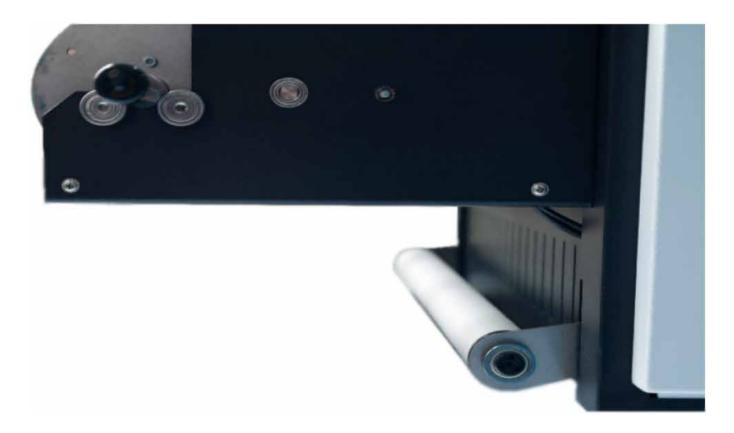
In **manual mode**, the roll function is activated, requiring the user to wrap the baked film from the bottom of the tension bar to the winding axis and secure the film with tape. The machine controls the speed of the winding according to the tension sensor.
