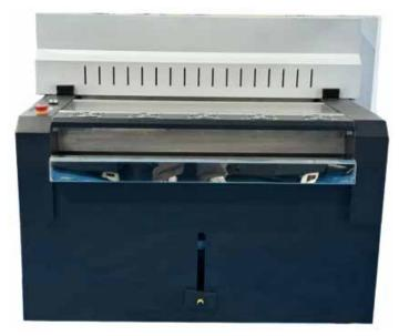
After activating Heating, the front preheating plate heating function will automatically turn on.
