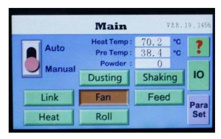
When using the **manual mode**, the vacuum roller function is activated, attaching the film to the Vacuum roller, pressing Fan once more this function will stop being used.
