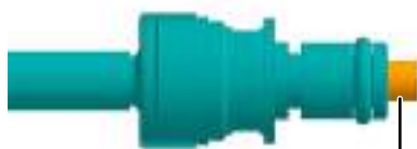
Valve not pushed in (valve sealed)
