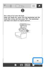
After oiling, insert the bobbin case into the hook, and then close the hook cover. (page 37)
