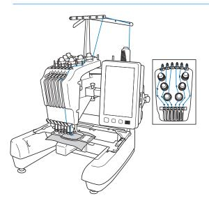
On the spool pin 1, place a spool with the thread color specified for the spool pin 1.
