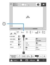
① Time until the machine stops
