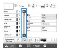
→ Each time is touched, the thread color sequence display scrolls down to the next color. After reaching the last color in the thread color sequence display, the first color is selected.
