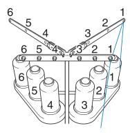
Pass the thread through the number 1 hole in the thread guide just above the spool, and then pass the thread through the number 1 hole in the thread guide toward the front of the machine.
