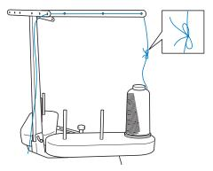
Pull out the old thread just after the needle bar thread guide.
