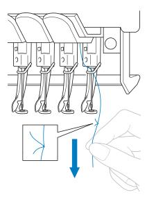
Continue pulling the thread until the knot is below the needle. Cut the knot.
