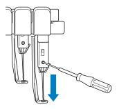
→ The needle and presser foot are locked in the down position.
