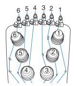
Pass the thread through the hole in the number 1 upper thread guide and pull the thread toward you.
