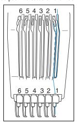
Pass the thread along the number 1 slot to pass it through the number 1 take-up lever hole from right to left
