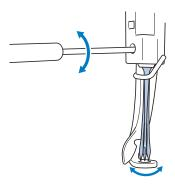
With the flat side of the needle toward the back of the machine, insert the needle all the way up until it touches the needle bar stopper.
