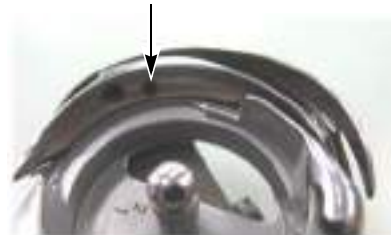
Lubrication hole (red mark)
