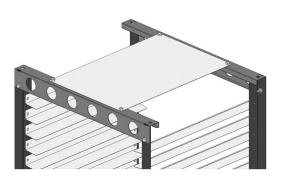
Install brace plate onto top and bottom of Screen Rack using 3/8" bolt and serrated nut. **Tighten well** with 9/16" wrench.
