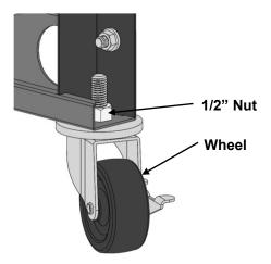
Install (4) wheels onto bottom of Screen Rack using 1/2" nut. **Tighten well** with 3/4" wrench. Once all wheels are installed, stand up the entire assembly.
