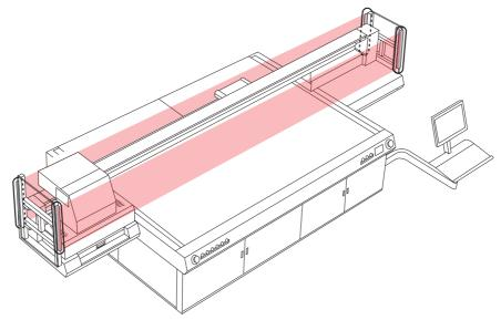
When all the following conditions are met, safety protection stops the machine.
