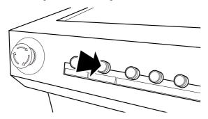
Press the [Vacuum Area] button to turn on the vacuum corresponding to the position the object to be printed on is in place.
