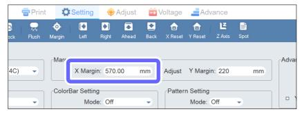
3 Enter the printing-start position on the Y axis to [Y Margin] in [Margin Setting].
