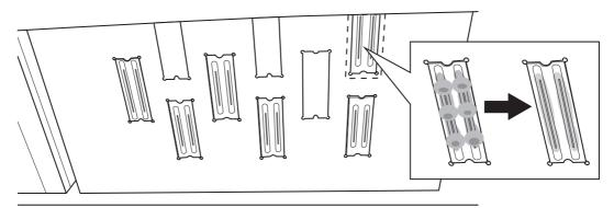
Clean the GI print head nozzle surface using new cleaning sticks.
