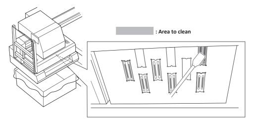
After cleaning, determine if the negative pressure value is set appropriately by checking the print head nozzle surfaces.
