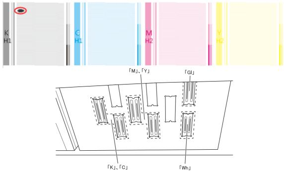
Adjust the negative pressure of the print head for which ink dropping is occurring.
