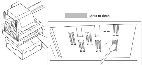
Repeat steps 4 to 9 to clean the print head nozzle surfaces using new cleaning sticks.
