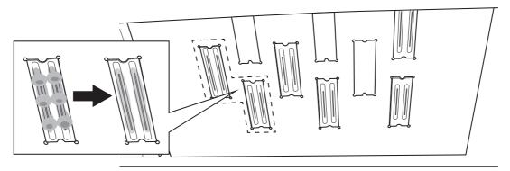
**6** Clean the K and C print head nozzle surfaces using new cleaning sticks.
