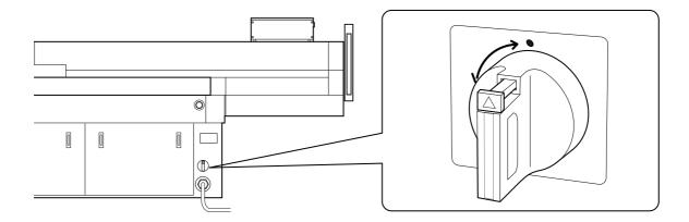
Check that the print-head carriage has returned to the maintenance station before turning off the power.
