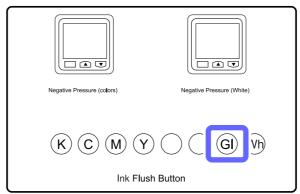
**8** Clean the GI print head nozzle surface using new cleaning sticks.
