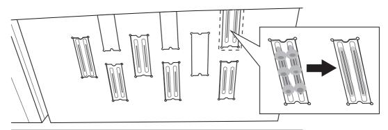
**8** Clean the GI print head nozzle surface using new cleaning sticks.
