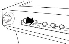
Press the [Vacuum Area] button to turn on the vacuum corresponding to the position the object to be printed on is in place.
