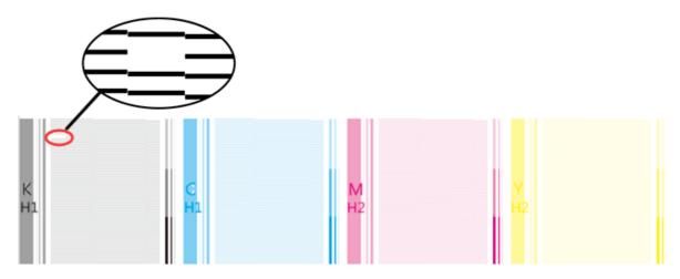
When printing is complete, check that no dot drop-out or dot displacement has occurred. If the problem persists, try performing head cleaning again. If the printer has been used for a long period, dot drop-outs may not be fixed even after performing head cleaning two or three times. If this is the case, perform liquid cleaning.
