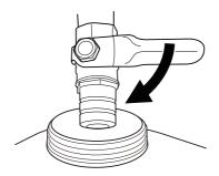
Turn the drain cock in the direction indicated with the arrow to close it.
