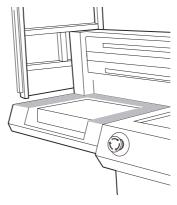
**4** Move the print-head carriage onto the maintenance station by pressing [Left] and [Right] on Print Exp.
