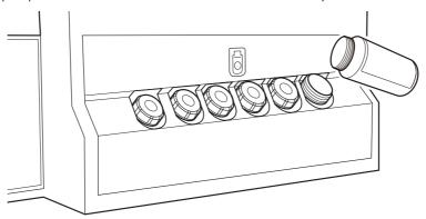
Tighten the cap on the ink tank.
