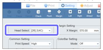
Enter the printing-start position on the X axis to [X Margin] in [Margin Setting].
