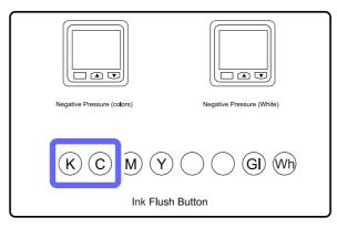
6 Clean the K and C print head nozzle surfaces using new cleaning sticks impregnated with cleaning liquid.
