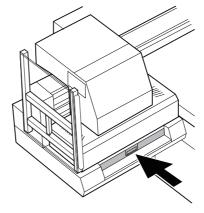
Clean the areas shown in the figure below using new non-woven fabric impregnated with cleaning liquid.
