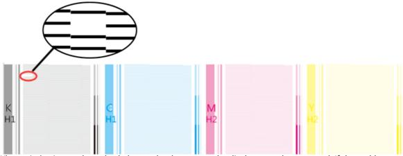
When printing is complete, check that no dot drop-out or dot displacement has occurred. If the problem persists, try performing head cleaning again. If the printer has been used for a long period, dot drop-outs may not be fixed even after performing head cleaning two or three times. If this is the case, perform liquid cleaning.
