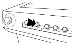
Press the [Vacuum Area] button to turn on the vacuum corresponding to the position the object to be printed on is in place.
