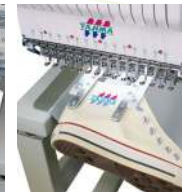
▲Air type Pocket Frame 2 (90mm x 30-258mm)
