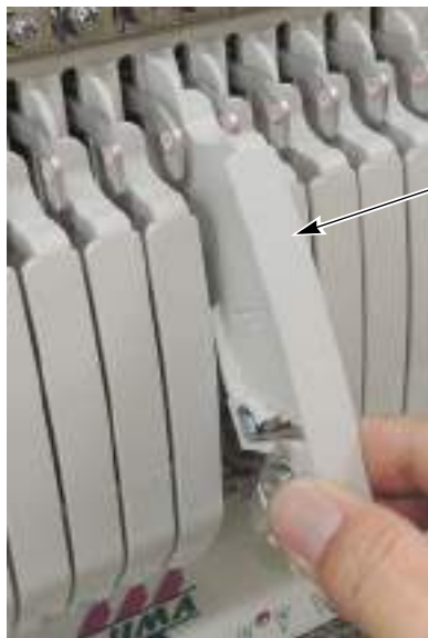
Snap-fit middle thread guide
