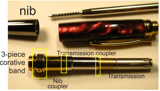
My suggested first option: Use some threadlock and carefully assemble the parts as shown. All of the yellow boxes have a junction that can be made relatively permanent, since the pen refill can be put into the pen by simply unscrewing the nib from the "gold part".
