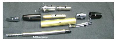
Before beginning assembly, make certain there is no glue remaining in the ends of your tubes. The first half inch of each end MUST be CLEAN. Use a small penknife or a round file to clean it out thoroughly!!! (I know I said this before, but it IS IMPORTANT!!!!!!!)
