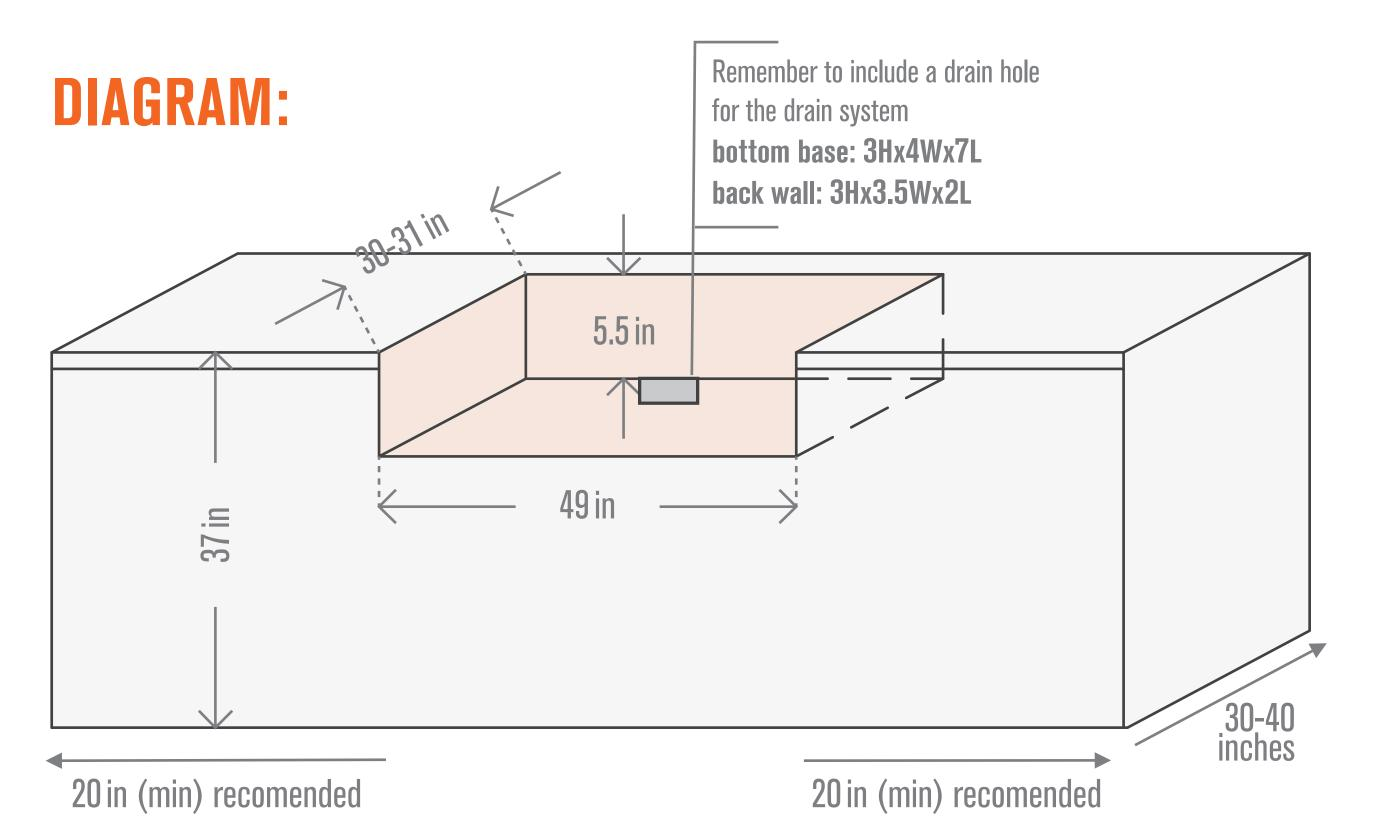
Please note, these measurements and diagrams are a recommendation only, and are estimated, for reference only. Dimensions may vary slightly because these products are hand finished. Always have the grill present while building the design and corroborate dimensions.
