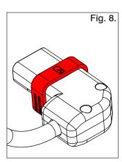
Replace the cord grip (Fig. 7.) ensuring the torque value is achieved (0.3Nm), and then replace the outer housing, screws and handle (Fig. 8.).
