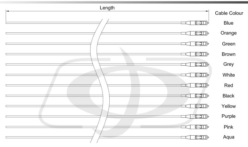
Length Tolerance: ±20mm(Length<0.5M). -0/+50mm(0.5M≤Length<1M). -0/+100mm(1M≤Length<10M). -0/+1%(Length≥10M).
