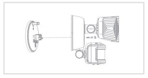
Connect the source wires from the outlet box with the wires of the back plate using wire nuts as follows:
