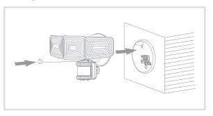
Using silicone caulking compound, caulk completely around where the light fixture meets the wall surface to prevent water from seeping into the outlet box.
