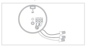
Place the back plate against the outlet box, insert the mounting bracket screw through the back plate hole, thread mounting bracket screw into the center hole of the mounting bar. Tighten the mounting bracket screw securely.
