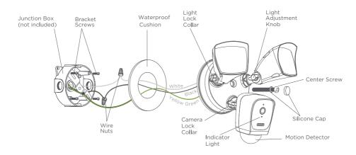
Europe/Australia gauge power cord color: Blue, Brown, Yellow green. Connect Floodlight Camera cables with same color junction box cables.
